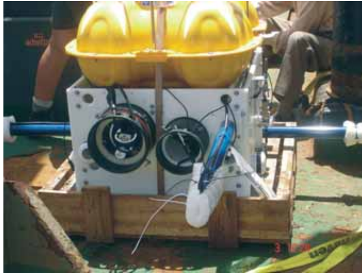
Fig.9. Marine MT equipment of Scripps Institution of Oceanography, San Diego used in Gulf of Kutch region. This is the first ever experiment using marine magnetotelluric technique in India.
