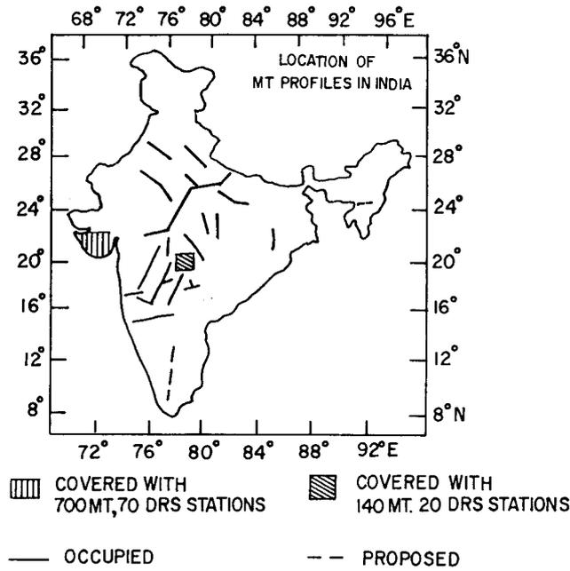
Figure 10. Compilation of location of wide band MT profiles by different organizations and institutions in India. The DRS stations are widely distributed in peninsular India and are not shown in the figure. Joint inversion applied to both the data sets near a deep bore hole in Saurashtra region is shown in Figure 6.
