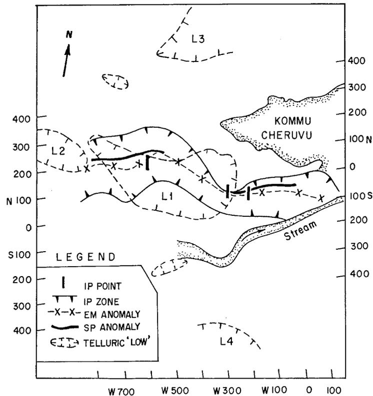
Figure 9. Integrated geophysical studies showing the anomalous conductive zones, near the Kalava area, Kurnool, India. Correlation of IP, SP, EM and telluric anomalous conductive zones interpreted as a deeper source of mineralization associated with carbonaceous shales. The numbers shown on the axis are distance in meters (from Harinarayana and Sarma, 1998a).
