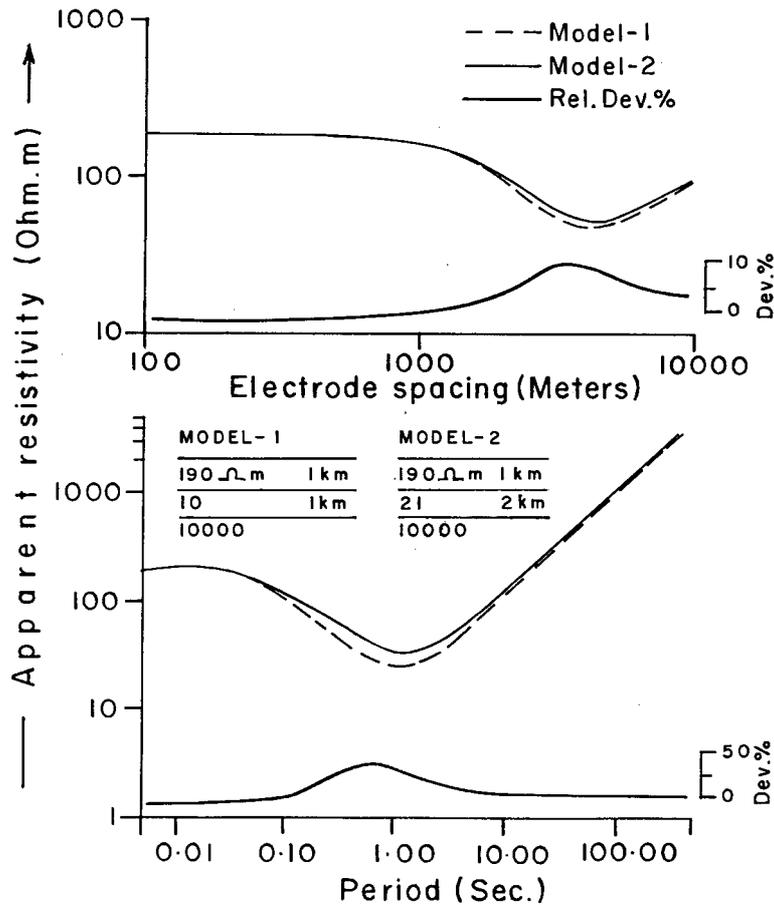
Figure 1. DC and MT apparent resistivity curves for two models and their relative deviation with respect to Model 1. Due to an equivalence problem, there is a small deviation in DC (top) and for the same model there is a large deviation for MT (bottom).
