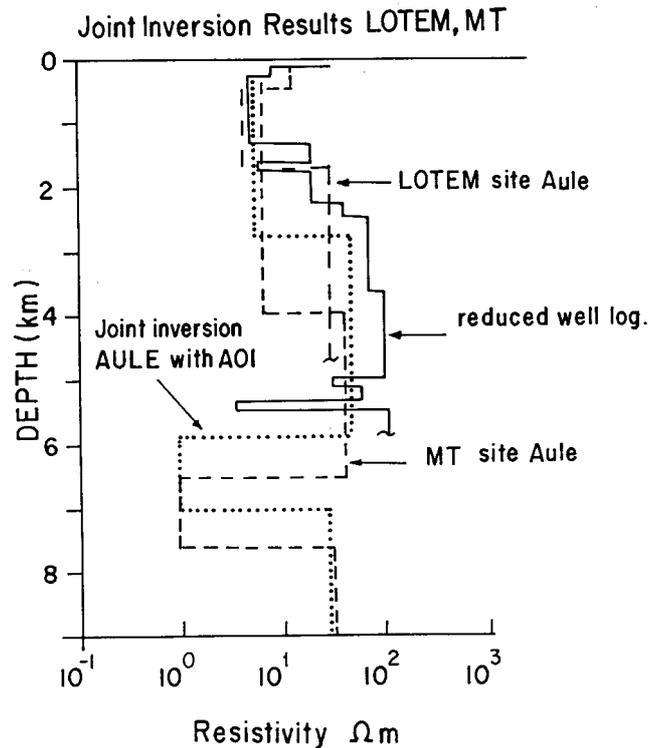
Figure 4. The results obtained from individual and joint inversion of MT and LOTEM datasets from NW Germany are compared with borehole laterolog (reduced) data. Joint inversion results are close to the bore hole data, (from Strack, 1992; originally from Hördt, 1989).
