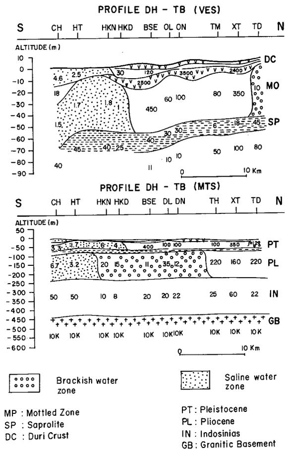
Figure 14. Near Ho Chi Minh City, Vietnam (top figure) derived from DC electrical sounding and from MT data (bottom figure). The sections are derived from simultaneous interpretation of both MT and DC data sets in an interactive mode with shallow section mainly from DC data and the deeper section both from MT and DC data (from Pham et al., 1994).
