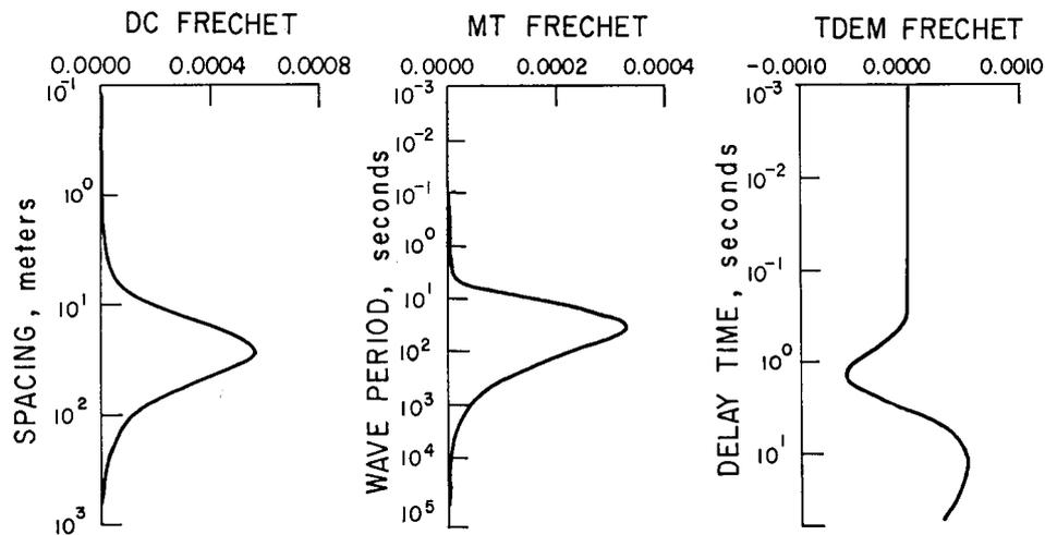
Figure 2. Frechet derivative curves for DC, MT and TDEM sounding methods. The shape and amplitude of the curves are similar for DC and MT with depth of burial, whereas TDEM curves are different (from Keller, 1992).
