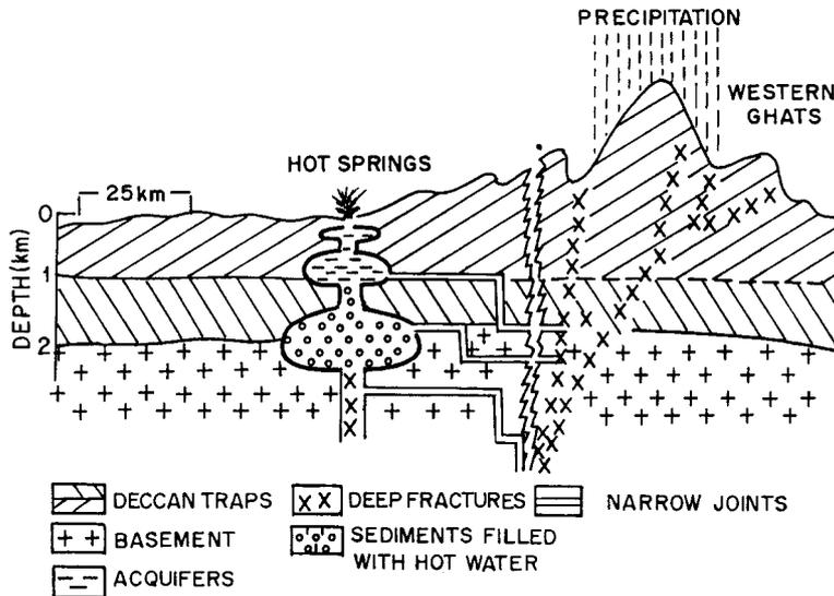
Figure 11. A schematic geological section is proposed based on shallow DC resistivity soundings, telluric and magnetotelluric data for Konkan geothermal province, west coast of India. DC resistivity soundings gave information on shallow aquifers and deep aquifers (1.5–2 km) is inferred from telluric and magnetotelluric studies (from Harinarayana and Sarma, 1998b).
